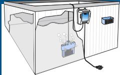
Install the [Saltron Mini](#) salt cell/chlorine generator per the manufacturer's instructions. The cell should be inspected every 3 months for scaling deposit. If scale exists, the cell should be cleaned with diluted [Acid Magic](#) per manufacturer's instructions.
